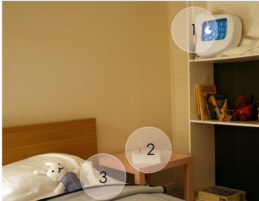
Figure 1: Reverse alarm clock elements (1) sky display, (2) treasure chest music box, (3) sensorial bed
